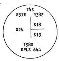
Brass washer nailed to B.T.blaze. Used stgel tape and magnetic compass with 18 East declination. Measured to center of all B.T.s
