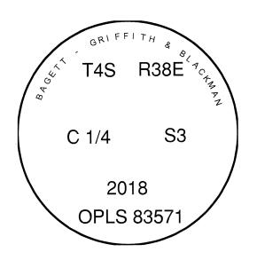
I used a Leica GS 15 GPS unit in the establishment of the new accessories. Basis of Bearing is as per map of survey number 016-2018. Distances and bearings are to the center of the 1  $\frac{1}{2}$ " aluminum caps.
