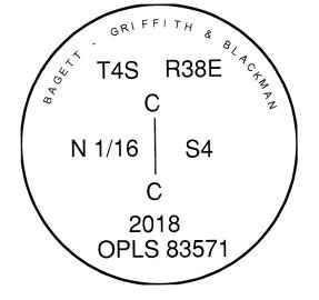
I used a steel tape and magnetic compass in the establishment of the new accessories. I used 13° East declination, the distances are to a 60d spike driven into the right side of the root crown of the bearing trees. A brass washer marked OPLS 83571 is attached to the BT blaze of the new bearing trees.
