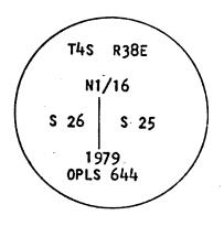
Brass washer nailed to B.T.blaze Used steel tape and magnetic compass with 18 East declination.
