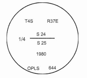
I used a steel tape and magnetic compass in the establishment of the bearing trees. Magnetic declination used was 13° East. Bearings are to a brass washer marked OPLS 83571 in the lower blaze of the new trees. Distance is to a spike set in the root crown of the side of the new trees.
