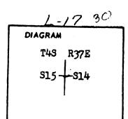
We found a stone of the correct size but cound not find the markings. A slab from a tree lays N40°W at 68 lksw marked with scribe # BT. A pine 32" in diam bears S40°E 57 lks with scribe visible.
