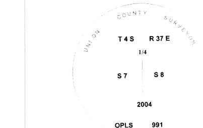
I used a steel tape and magnetic compass in the establishment of new accessories. The magnetic declination used was 18° East. The distance to the bearing trees are to a 50d spike driven on the right side of the tree at the root crown. I attached a brass washer marked OPLS 991 to the BT Blaze
