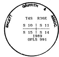
I used a steel tape and magnetic compass in the establishment of new accessories. I used 17° magnetic declination. The distances are to a 50d spike driven in the right side of the root crown. I attached a brass washer marked OPLS 991 to the BT blaze.
