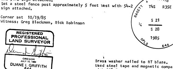
Brass washer nailed to BT blaze. Used steel tape and magnetic compass with 20° East declination. Measured to 50d spike set in right side of tree when facing tree, unless otherwise stated.
