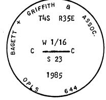
Brass washer nailed to BT blaze. Used steel tape and magnetic compass with 20° East declination. Measured to 50d spike set in right side of tree when facing tree, unless otherwise stated.
