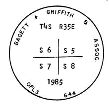
Brass washer nailed to BT blaze. Used steel tape and magnetic compass with 20° East declination. Measured to 50d spike set in right side of tree when facing tree, unless otherwise stated.
