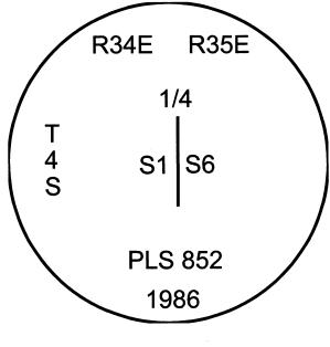
I used a steel tape and magnetic compass in the establishment of the new accessories. I used  $14^\circ$  East declination, the distances are to a 60d spike driven into the right side of the root crown of the bearing trees. A brass washer marked OPLS 83571 is attached to the BT blaze of the new bearing trees.
