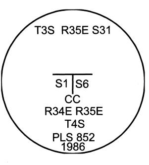
I used a steel tape and magnetic compass in the establishment of the new accessories. I used 14° East declination, the distances are to a 60d spike driven into the right side of the root crown of the bearing trees. A brass washer marked OPLS 83571 is attached to the BT blaze of the new bearing trees. Distances and bearings for the iron pins are to the center of the aluminum caps.
