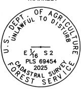
Placed a plastic-encased magnet at the base of the monument. Used RTK GPS to measure accessories. Bearings are geodetic, based on GPS observation at the corner. I set an aluminum post South, 2.0 ft. with 54-9 and 54-2 USFS signs attached and another one East, 26 ft. from the monument with 54-2 USFS sign attached.
