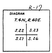
A spruce, 10 ins. diam. bears N 16° E, 23 lks. dist. mkd. T 4 N R 40 E S 23 BT. A spruce, 10 ins. diam. bears S 74° W, 24 lks. dist. mkd. T 4 N R 40 E S 27 BT. A tamarack, 20 ins. diam. bears N 57° W, 46 lks. dist., mkd. T 4 N R 40 E S 22 BT.
