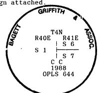
OREGON JULY 10, 1964 **DUANE I. GRIFFITH**  I used a steel tape and magnetic compass in the establishment of new accessories. I used 20° East magnetic declination and the distances are to the "+" chiseled on the bearing object.
