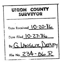
See map of survey number 29-86 filed in the Union County Surveyor office. Description of monument and accessories lestablished to perpetuate the original location of this corner: At position determined by survey, I set a 2½ ×30" aluminum pipe with aluminum cap marked as shown, 20 inches in the ground; From which:
