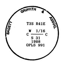
I used a steel tape and magnetic compass in the establishment of new accessories. I used 20° East magnetic declination and the distances are to a 50d spike driven in the right side of the root crown. I attached a brass washer marked OPLS 991 to the BT blaze.
