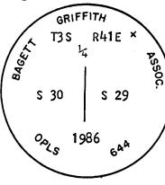
Brass washer marked OPLS 644 nailed to BT blaze. Used steel tape and magnetic compass with 20° East declination. Distances to the BTs are to a 50d spike set in right side of tree when facing tree, unless otherwise stated.
