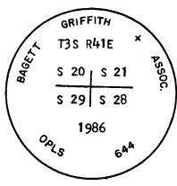
Brass washer marked OPLS 644 nailed to BT blaze. Used steel tape and magnetic compass with 200 East declination. Distances to the BTs are to a 50d spike set in right side of tree when facing tree, unless otherwise stated.
