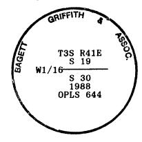
I used a steel tape and magnetic compass in the establishment of new accessories. I used 18° East magnetic declination and the distances are to a 50d spike driven in the right side of the root crown. I attached a brass washer marked OPLS 644 to the BT blaze.
