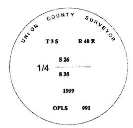
I used a steel tape and magnetic compass in the establishment of the new accessories. I used 18° East declination, the distances are measured to a 60d spike driven in the right side of the root crown.
