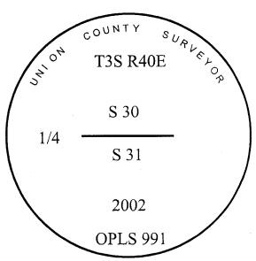
I used a steel tape and magnetic compass in the establishment of the new accessories. I used 18° East declination. The distances to the accessories are to the center of the aluminum cap.
