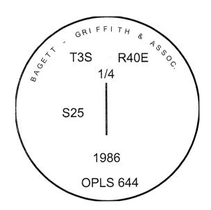
I used a steel tape and magnetic compass in the establishment of the new accessories. I used 15° East declination, the distances are to a 60d spike driven into the right side of the root crown of the bearing trees. A brass washer marked OPLS 2219 is attached to the BT blaze of the new bearing trees.
