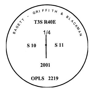
I used a Leica 530 GPS unit in the establishment of the new accessories. The Basis of Bearings is the same as that shown on Survey No. 024-2001. The distances are to the center of a 5/8"x30" iron pin with 1 ½" aluminum cap.
