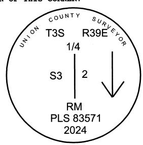
A 5/8" x 30" iron pin bears South 69°04' West, a dist. of 66.82 feet, with 1 1/2" aluminum cap marked UNION COUNTY SURVEYOR SW RP from true corner position (bears South 44°21' West, a dist. of 89.32 feet from reference monument).
