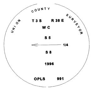
I used a steel tape and magnetic compass in the establishment of the new accessories. I used 17° East declination.
