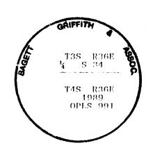
I used a steel tape and magnetic compass in the establishment of new accessories. I used 17° magnetic declination. The distances are to a 50d spike driven in the right side of the root crown. I attached a brass washer marked OPLS 991 to the BT blaze.
