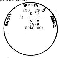
I used a steel tape and magnetic compass in the establishment of new accessories. I used 17° magnetic declination. The distances are to a 50d spike driven in the right side of the root crown. I attached a brass washer marked OPLS 991 to the BT blaze.
