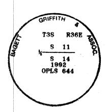
I used a transit and distance to accessaries and show inversed bearings and distances. Bearing and distances are to a 50d spike driven in the right side of the root crown. I attached a brass washer marked OPLS 644 to the BT blaze.
