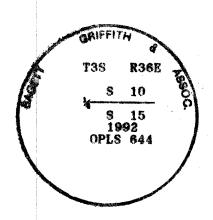
I used a steel tape and magnetic compass in the establishment of new accessories. I used 20° East magnetic declination and the distances are to a 50d spike driven in the right side of the root crown. I attached a brass washer marked OPLS 644 to the BT blaze.
