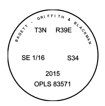
I used a steel tape and magnetic compass in the establishment of the bearing trees. Magnetic declination used was 15° East. Bearings are to a brass washer marked OPLS 83571 in the lower BT blaze. Distances are to at 60d spike in the right hand side of the tree.
