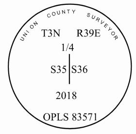
I use a RTK GPS in the establishment of the accessories. Bearings and distances are to the center of the aluminum caps. Basis of Bearing is as per Survey Number 002-2018.
