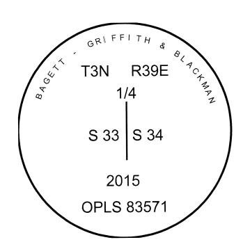
I used a steel tape and magnetic compass in the establishment of the bearing trees. Magnetic declination used was 15° East. Bearings are to a brass washer marked OPLS 83571 in the lower BT blaze. Distances are to at 60d spike in the right hand side of the tree.
