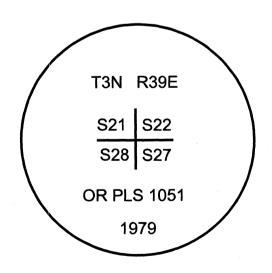
I used a compass and tape in the establishment of the new accessories. Bearings are to a brass washer marked OPLS 83571 in the BT blaze and distances are measured to a 60D spike in the right side of the center of the tree. I used 14° East for magnetic declination.
