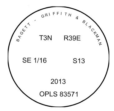
I used a Leica RTK GPS in the establishment of the bearing accessories. Basis of bearing is as per Survey Number 056-2013. Bearings and distances are to the center of the aluminum cap.
