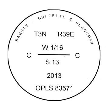
I used a steel tape and magnetic compass in the establishment of the bearing trees. I used 16° East declination, the distances are to a 60d spike driven into the right side of the root crown of the tree. A brass washer marked OPLS 83571 is attached to the BT blaze of the bearing trees.
