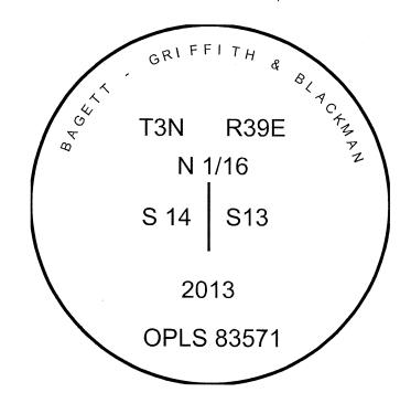
I used a steel tape and magnetic compass in the establishment of the accessories. Magnetic declination used was 16° East. Distances are to a 60d spike in the right hand side of the root crown of the trees. Bearings are to a brass washer marked OPLS 83571 in the BT blaze of the tree.
