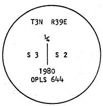
Brass washer nailed to BT blaze. Used steel tape and magnetic compass with 17°declination, East. Distance measured to
