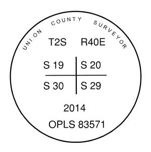
I used a Leica GS15 RTK GPS in the establishment of new accessories. The Basis of Bearings is the same as that of Survey No. 008-2014 The bearings and distances are The bearings and distances are to the center of the aluminum caps.
