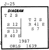
Corner MODIFIED by Alonzo Gesner under contract No.683 and dated June 07, 1898, and his records state: Found original post marked and witnessed as stated by the U.S. Surveyor General. I obliterated marks on the NE and SE faces of post, also obliterated marks on the bearing trees in Secs 7 and 18. I marked the NW face of post T 2 S.
