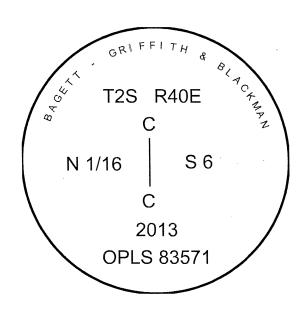
I used a steel tape and magnetic compass in the establishment of the new accessories. I used 16° East declination. The distances are to a 60d spike in the right hand side of the root crown of the new bearing trees. Bearings are to a brass washer marked OPLS 83571 in the lower BT blaze.
