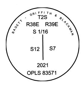
I used a Leica GS18 with RTK in the establishment of the new accessories. Bearings and distances are measured to the center of the aluminum cap. Basis of bearing is as per Survey Number 018-2021.
