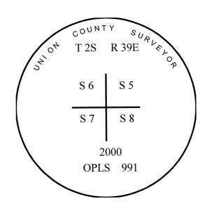
I used a steel tape and magnetic compass in the establishment of the new accessories. I used 16° East declination, the distances are to center of aluminum cap, unless otherwise noted.
