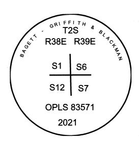
I used a Leica GS18 with RTK in the establishment of the new accessories. Bearings and distances are measured to the center of the aluminum cap. Bearings are to the power pole are to the center of the pole. Distances are to a spike in the side of the pole. Basis of bearing is as per Survey Number 018-2021.
