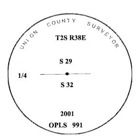
I used a compass and steel tape in the establishment of the new accessories. I used 18° East declination. The distances are to the center of a 5/8"x30" rebar with 1 ½" aluminum cap marked Union County Survey Marker.
