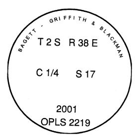
I used a total station instrument in the establishment of the new accessories. The basis of bearing is the same as survey number 042-2001. The distances are to a 60d spike driven into the right side of the root crown of the bearing tree. I attached a brass washer marked OPLS 2219 to the BT blaze.
