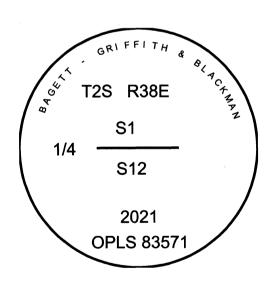
I used a Leica GS18 with RTK in the establishment of the new accessories. Bearings and distances are measured to the center of the aluminum cap. Basis of bearing is as per Survey Number 018-2021.
