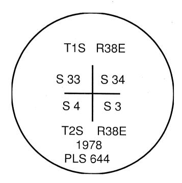
I used a Leica VIVA RTK GPS in the establishment of the accessories. Basis of bearings is as per Survey Number 004-2007. Bearings and distances are to the center of the aluminum cap.
