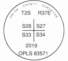
I used a steel tape and magnetic compass in the establishment of the new accessories. I used 13° East declination, the distances are to a 60d spike driven into the right side of the root crown of the bearing trees. A brass washer marked OPLS 83571 is attached to the BT blaze of the new bearing trees.
